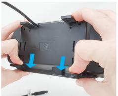
Next, place the monitor over the existing mirror, let go of the lower clips so that they clamp the monitor to the interior mirror.
